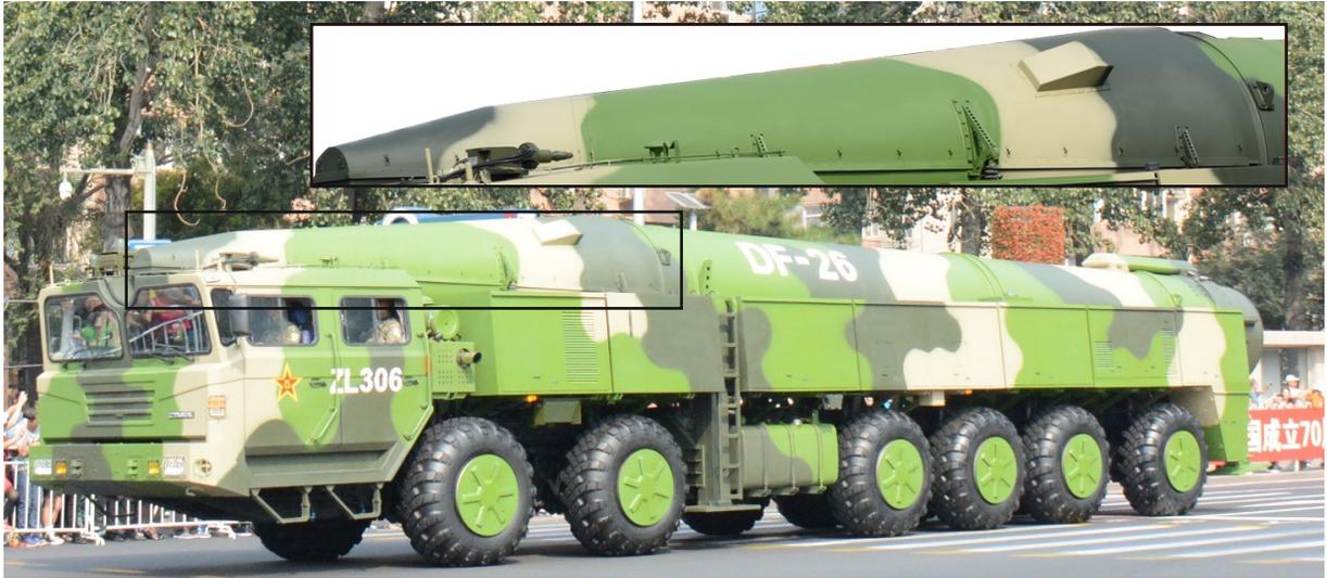
**DF-26 IRBM.** China continues to field the dual-capable DF-26 IRBM that constitutes its first ever precision-strike nuclear capability. The comingling of nuclear and conventional capabilities raises the potential for inadvertent escalation during a conflict. Note the hinged payload access compartment, (inset) which is unique among China's nuclear capable systems. | Image Source: DoD
