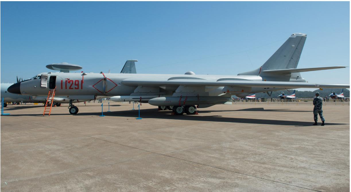
**Building Air Based Nuclear Capabilities.** The improved H-6N bomber constitutes the nascent air leg of China’s nuclear triad. Distinct from the H-6K pictured above and other variants, the H-6N has an air-to-air refueling capability and a recessed fuselage that can carry a nuclear armed air-launched ballistic missile. China intends to surpass this capability with the H-20 stealth strategic bomber that is under development.
