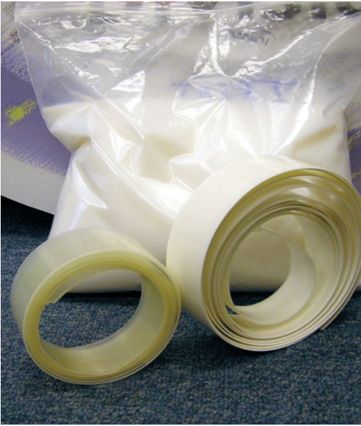
As part of its experimentation, the team at Kennedy melted down some of its aerogel-infused plastics and extruded them into tapes. Credit: NASA
