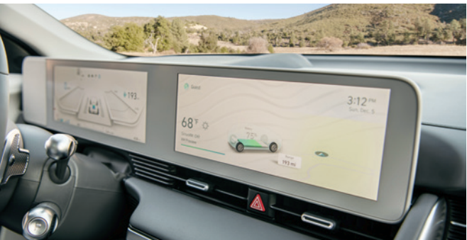
Since 2020, the interfaces on the infotainment and instrument cluster displays on Hyundai car models have been produced with DiSTI’s GL Studio software. The ability to run on this sort of integrated hardware can be traced back to requirements for NASA. Credit: Hyundai Motor America
