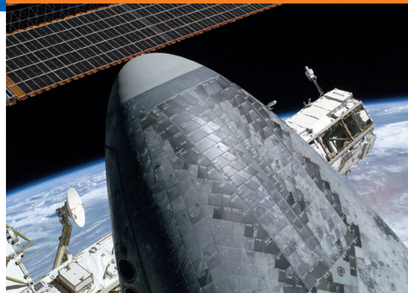
This picture of the underside of the space shuttle Discovery's nosecone shows the thermal protection system (TPS) tiles that Canopy Aerospace now manufactures. Credit: NASA
