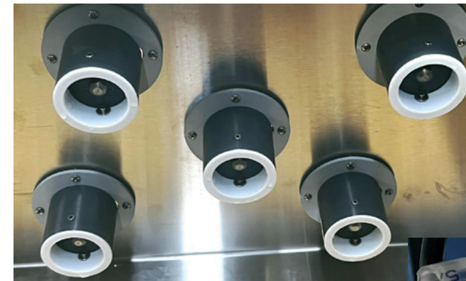
Electrostatic spray nozzles impart a small electric charge to minuscule particles of water, allowing the droplets to stick to surfaces. This array of sprayers, made by Electrostatic Spraying Systems (ESS), is used in food production. Credit: Electrostatic Spraying Systems Inc.
