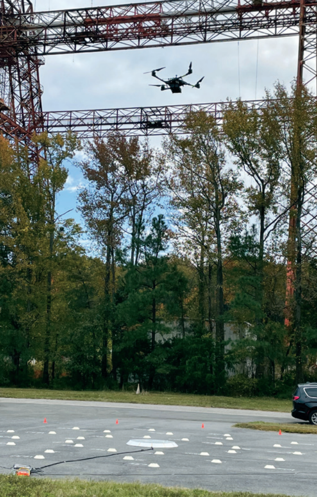
The WirelessArray developed by IC2, laid out here for a test flight at Langley Research Center, makes flight testing for drones quick and cost-effective. Credit: NASA
