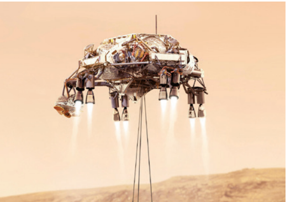
As the sky crane descended toward Mars at approximately 200 mph, eight engines fired to produce a counterthrust to reduce its speed to about 1.7 mph before lowering the rover to the surface. Eaton developed a custom pyrovalve to ensure the fuel was released at just the right moment. Credit: NASA/JPL-Caltech
