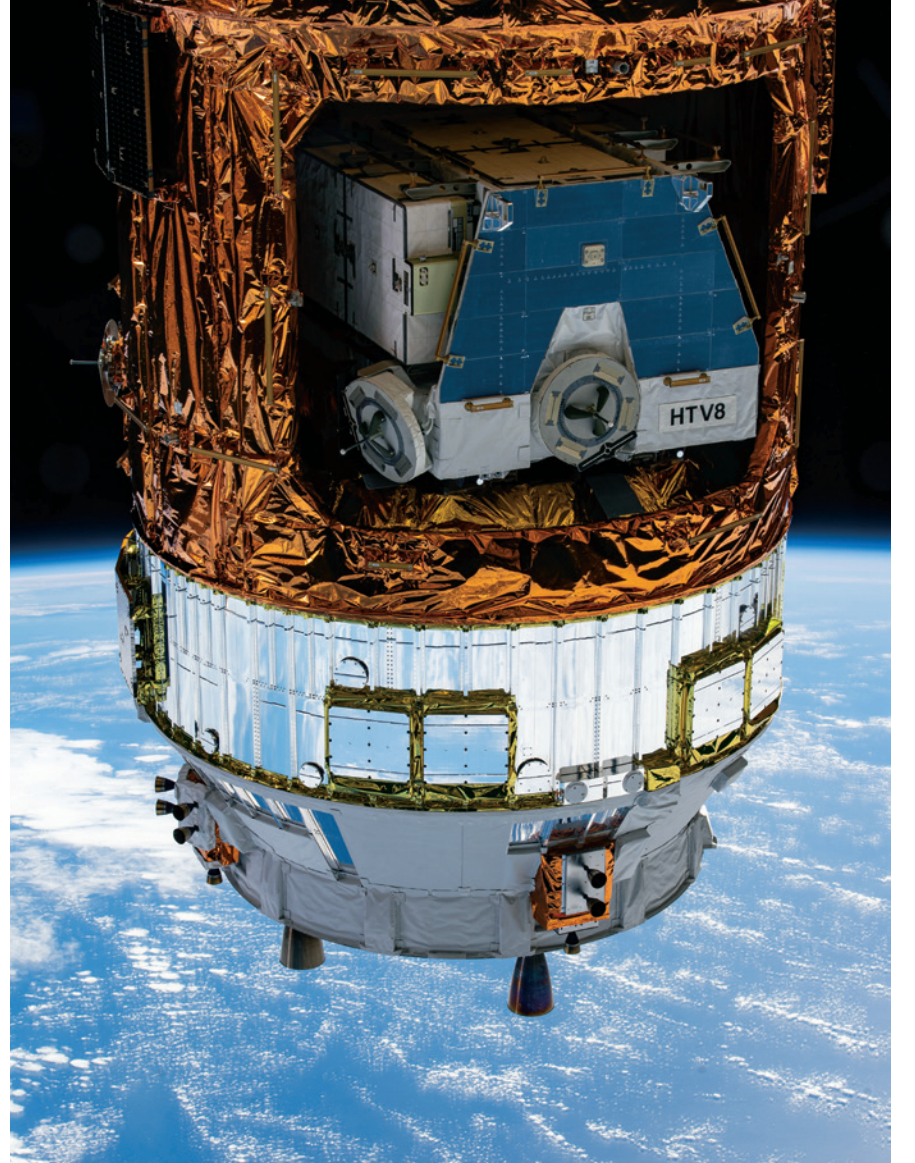
Nickel-hydrogen batteries were the primary energy storage for the International Space Station for more than 18 years before being replaced and, pictured here in 2020, returned to Earth. Credit: NASA
