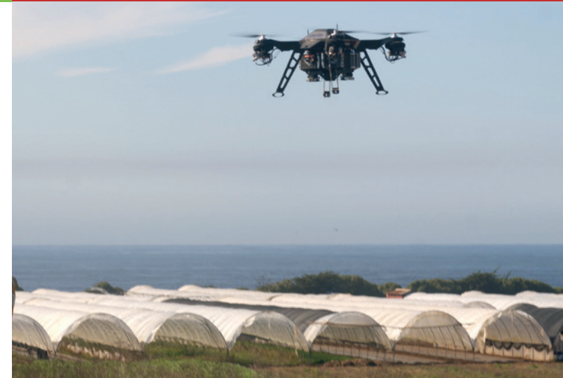
Parallel Flight Technologies' Firefly aircraft is designed to run for 100 minutes while fully loaded, allowing the aircraft to perform agricultural surveys as well as assist in the aftermath of natural disasters. Credit: Parallel Flight Technologies Inc.
