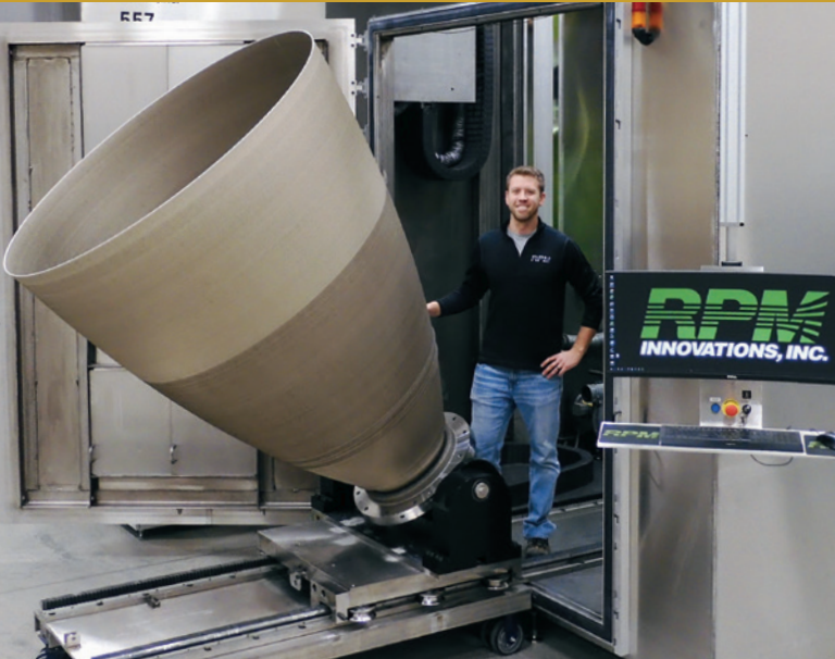
Tyler Blumenthal, sales manager at RPM Innovations, stands with a 3D printed rocket engine nozzle, freshly printed using the technique the company refined with NASA for large-scale metal 3D printing. At about five feet across and six-and-a-half feet tall, this is a 65% scale model of the nozzle from the RS-25 engines that were the space shuttle main engines and now power the SLS's (Space Launch System) core stage. Credit: RPM Innovations Inc.
