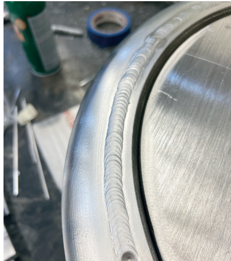
This 3D printed aluminum nozzle was then welded with wire from Elementum 3D spinoff Fortius Metals. Credit: NASA
