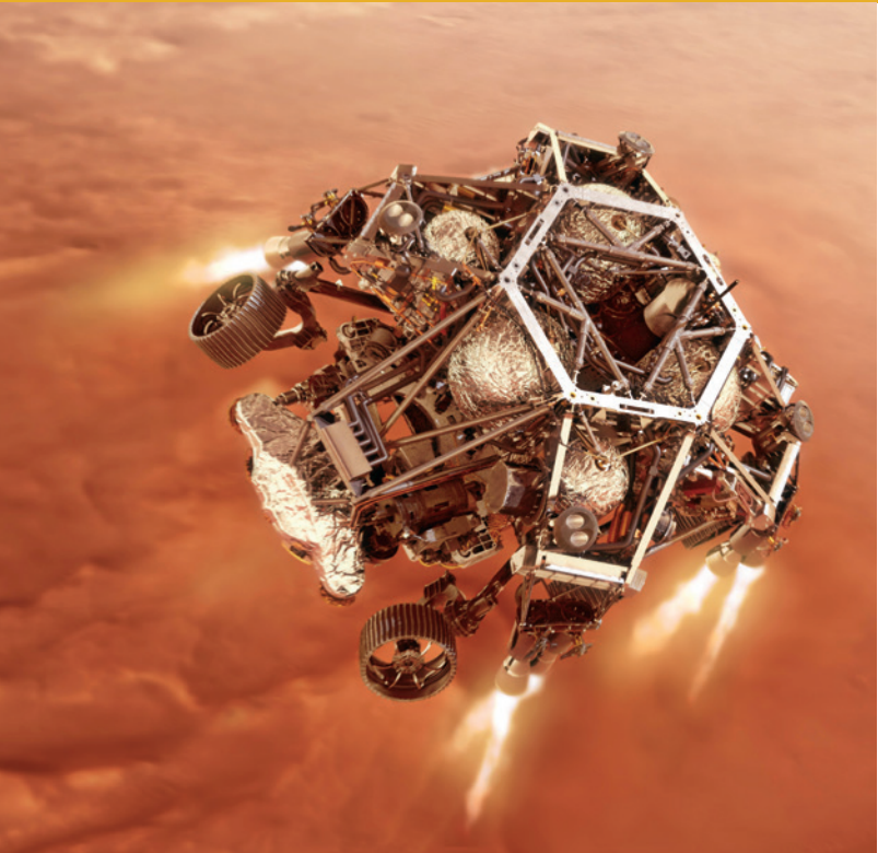
The controlled descent of the Mars Curiosity rover included the use of propulsion rockets pointing to the surface to allow a gentle landing. The engine, shown firing in this illustration of Perseverance and the sky crane landing system relied on a pyrovalve that released the rocket fuel. Credit: NASA/JPL-Caltech
