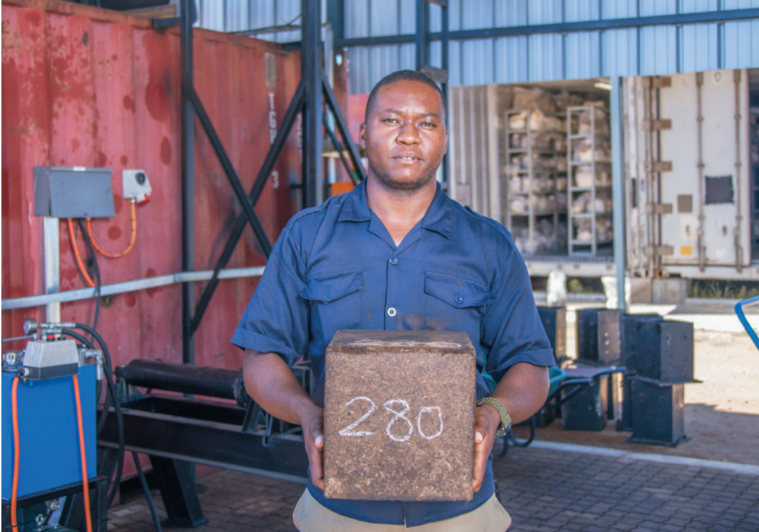
Ivan Severus, site manager for Mycohab, holds a brick made from substrate used to grow mushrooms. This mycomaterial comes from woody mulch bound together by the fungal mycelia. Credit: Mycohab Ltd.
