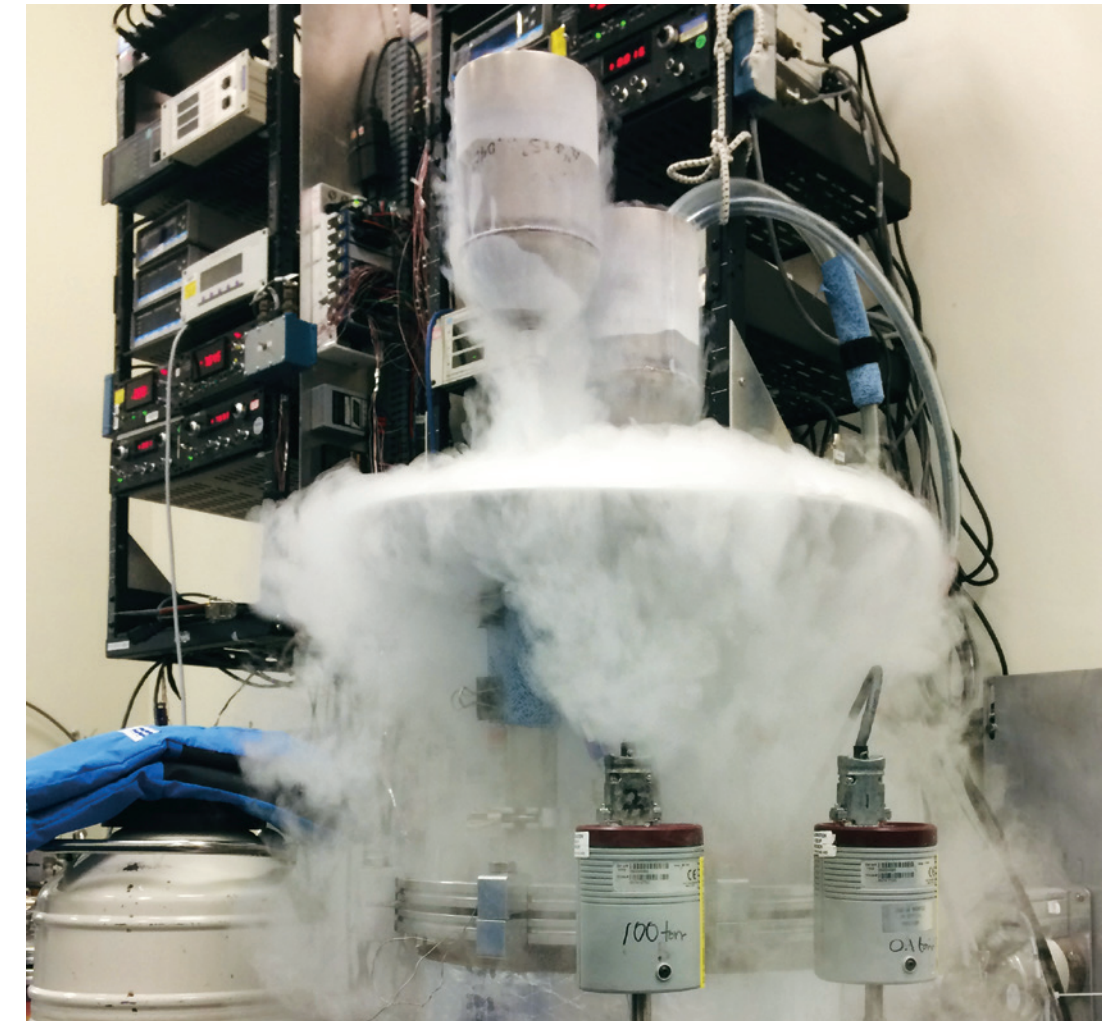
NASA's Cryostat CS-500, pictured here as it cools down to cryogenic temperatures, was developed by GenH2 cofounder James Fesmire when he headed the Cryogenics Test Laboratory at NASA's Kennedy Space Center. Credit: NASA
