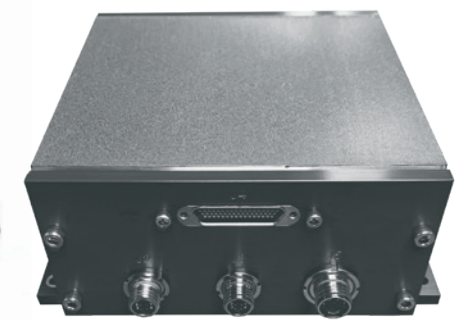
AFTU hardware tested by NASA's Flight Opportunities program (left) replaces the human decision-making step required to assess any problems a rocket might have and then send a destruct command. Sagrad helped build the technology and now sells smaller, cheaper versions—the original AFTU (center) and the new Integrated AFTU (right). Credit: NASA (left), Sagrad Inc. (center, right)
