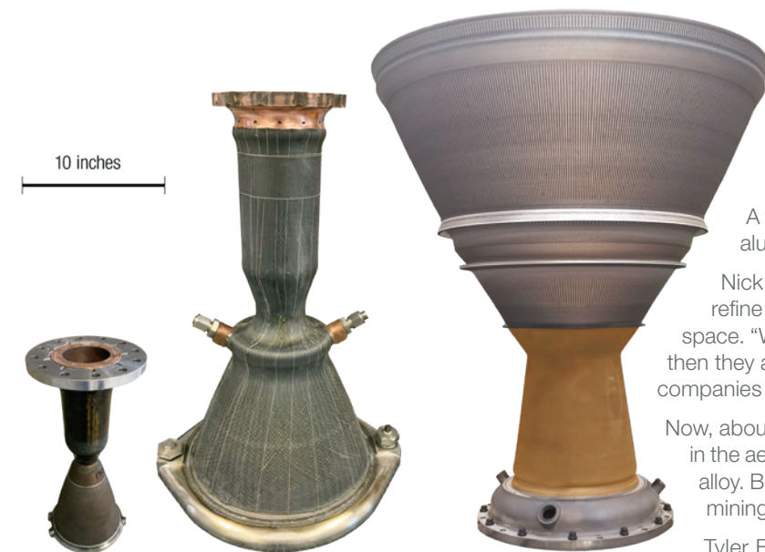
Under the Rapid Analysis and Manufacturing Propulsion Technology program, RPM Innovations and NASA 3D printed different classes of rocket engine thrust chambers to mature the novel technologies associated with each. Seen here are the printed engines capable of 2,500, 7,000, and 40,000 pounds of thrust. Credit: NASA
