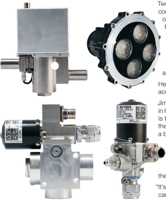
Marotta Controls developed these valves as a subcontractor to NASA’s Commercial Resupply Services and Commercial Crew programs and now sells them to other commercial launchers. Clockwise from top left: The MFV400 electronic pressure regulator is now on a commercial lunar lander. The PRV15B negative pressure relief valve prevents capsules from being crushed on atmospheric reentry. The MV100X is used in small thrusters to adjust spacecraft orientation. And the MV524 controls flows from pressurized tanks. Credit: Marotta Controls Inc.
