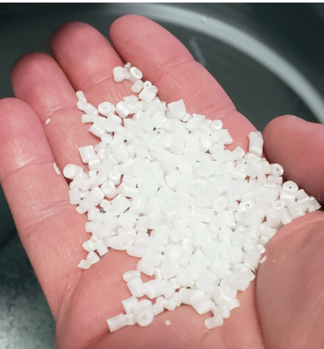
Okhata customers purchase aerogel-infused plastics, or “aeropolymers,” as tiny pellets and then melt them down to manufacture products, usually through injection molding or extrusion. Credit: Aeropolymer Holding Group
