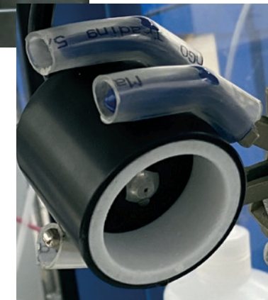
An ESS mister nozzle undergoes testing at Kennedy Space Center. The design was improved through collaboration between the company and NASA. Credit: NASA
