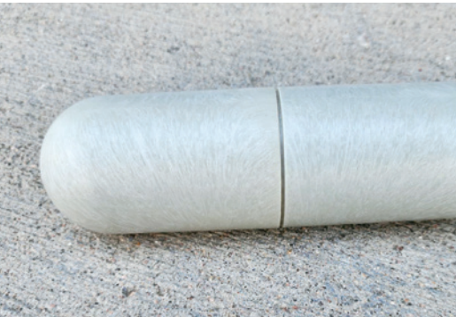
Another Okhata customer made this case from an aeropolymer to test the material’s thermal insulation properties. Credit: Aeropolymer Holding Group
