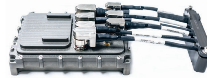
AFTU hardware tested by NASA's Flight Opportunities program (left) replaces the human decision-making step required to assess any problems a rocket might have and then send a destruct command. Sagrad helped build the technology and now sells smaller, cheaper versions—the original AFTU (center) and the new Integrated AFTU (right). Credit: NASA (left), Sagrad Inc. (center, right)
