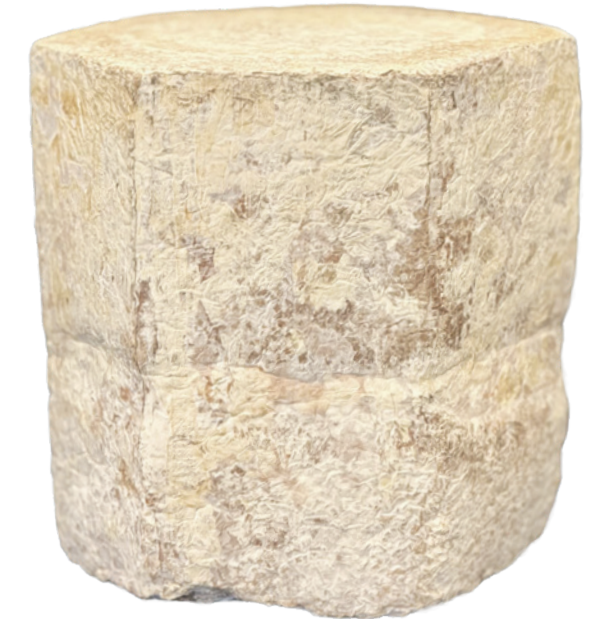
This stool created by a NASA-funded project proves it's possible to fabricate furnishings using the same fungal mycelia that create bricks on Earth. Credit: NASA
