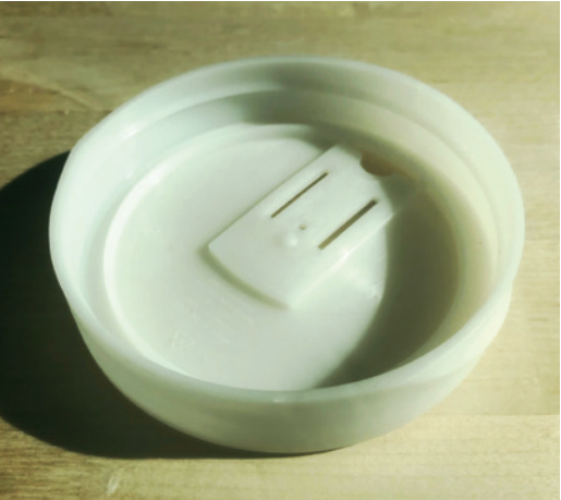
One Okhata customer used an aeropolymer to produce a beverage lid that is insulative and doesn’t let liquid cling to it. Credit: Central Custom Molding LLC
