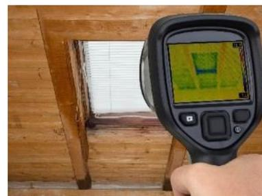
**Figure 9.** A thermal imager being used indoors to assess windows for leaks.
