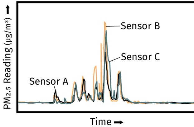
Sensor C does not appear to track concentration in the same way as sensors A and B. This could be problematic.
