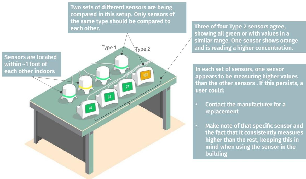
**Figure A4-1.** An example set up for how to perform a sensor “precision check” prior to deploying multiple sensors in a space.
