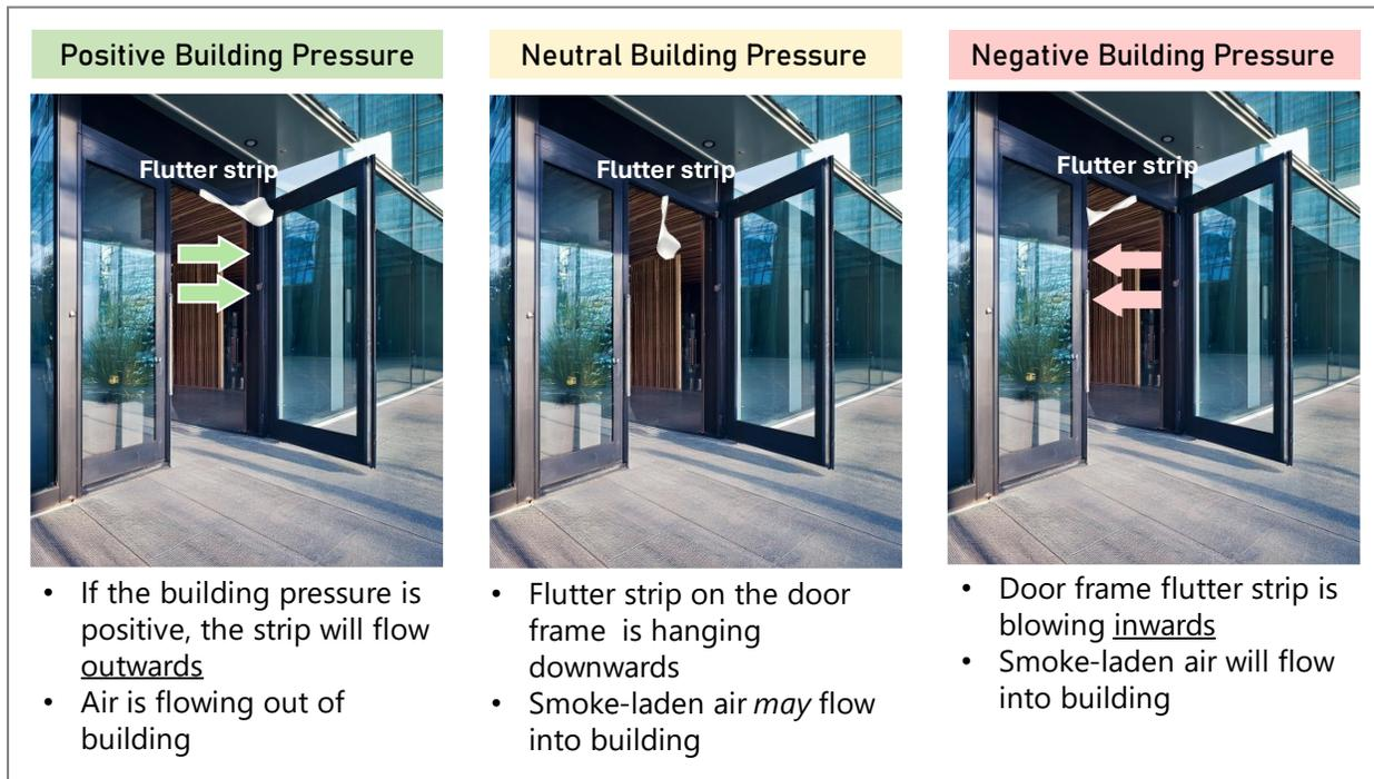
**Figure 6.** Examples of flutter strip test results under different building pressure scenarios.
