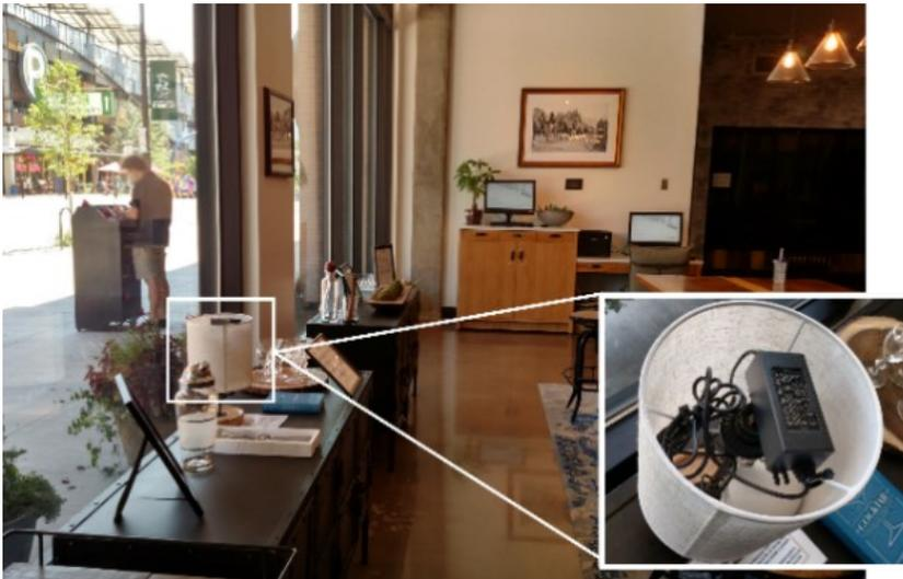
**Figure 16.** A camouflaged indoor air sensor. The sensor is in populated hotel lobby where air can flow into and around the sensor. Placing it inside a non-functional lamp shade keeps it out of sight.
