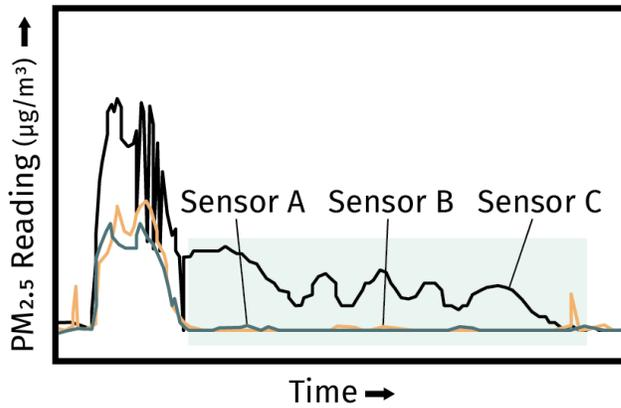
**Figure A4-3.** An example of sensor data that track appropriately (top), and an example where one sensor is exhibiting problematic behavior (bottom).
