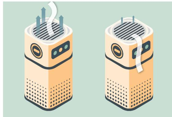
**Figure 13.** (Left) a PAC with a flutter strip exhibiting air flow and (Right) reduced air flow
