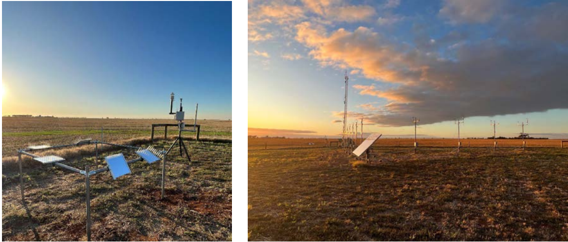
Figure 24. Soiling Rig at the Atmospheric Boundary Layer Research Facility
