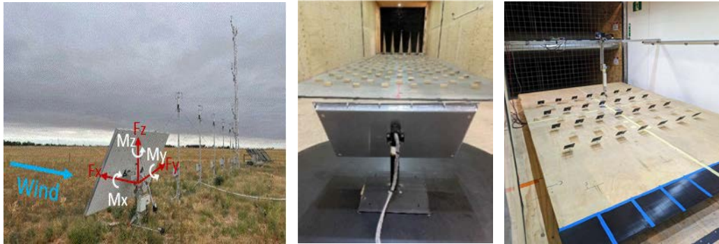
Figure 23. Experimental setup and instrumentation for heliostat wind load measurements at the University of Adelaide Atmospheric Boundary Layer Research Facility (ABLRF) and wind tunnel
