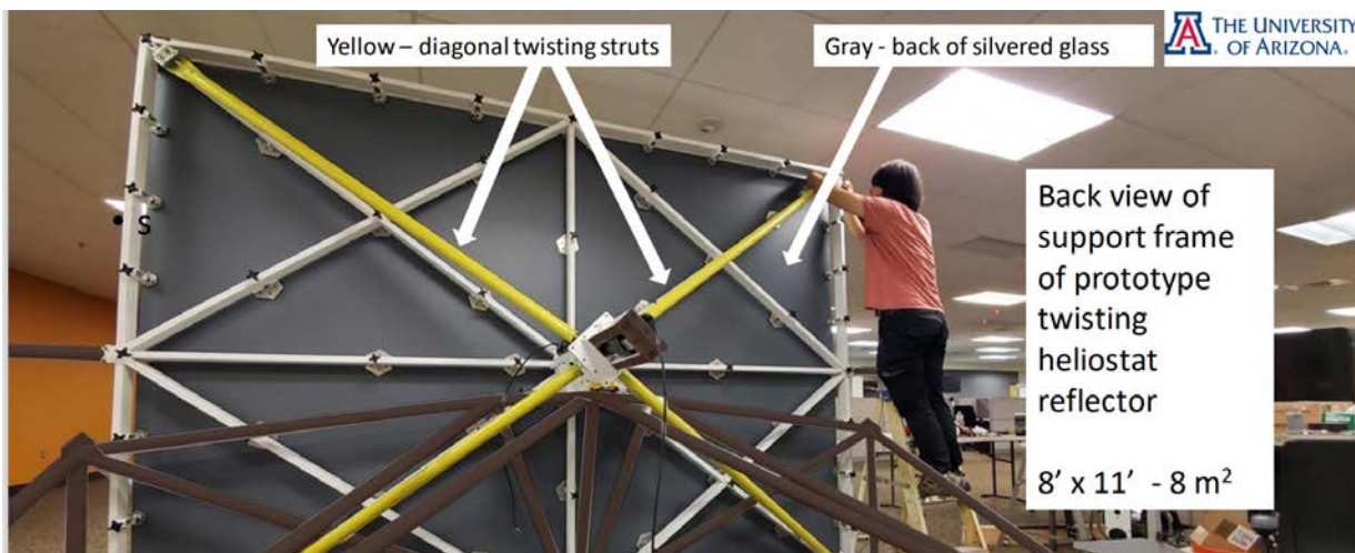
Figure 20. Prototype of high-performance twisting heliostat
